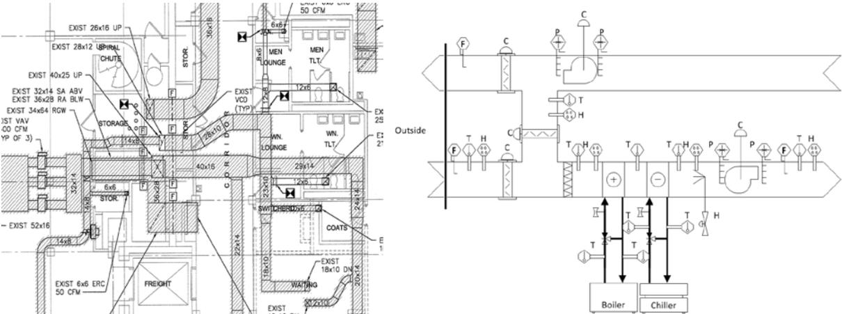
Figure 2 Examples of mechanical plan drawing (left) (a section of mechanical plan of a campus building) and P&ID drawing (right) (adopted from Sugarman (2005))
