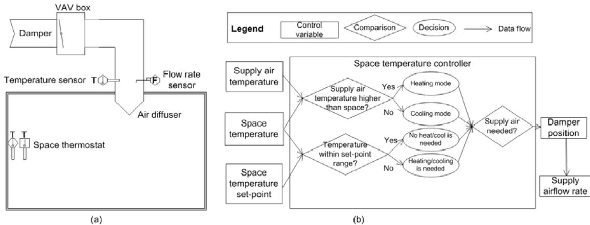
Figure 3 An example of a local control loop that adjusts the temperature of a space, where (a) shows the P&ID drawing and (b) shows the data flow in this control loop
