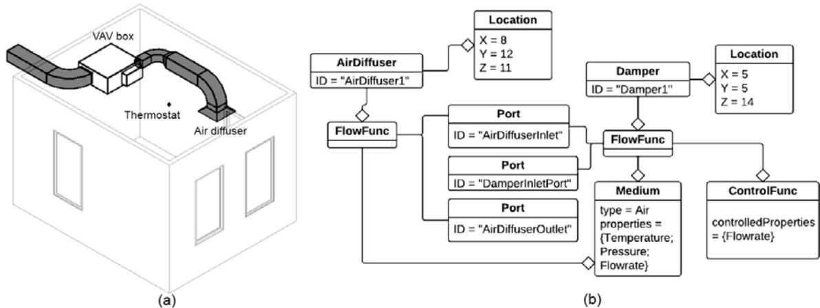
Figure 5 (a) Screenshot of the Revit model used in the prototype; (b) Examples of the implementation of proposed taxonomy
