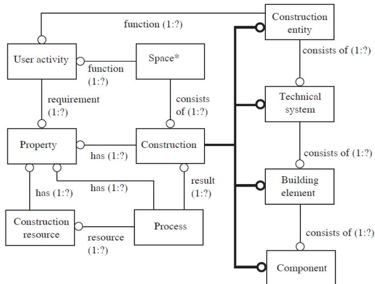
Figure 4. A conceptual model of the built environment reflecting certain information described in ISO 12006-2. The asterisk marks that Space is defined by spatial relations.
