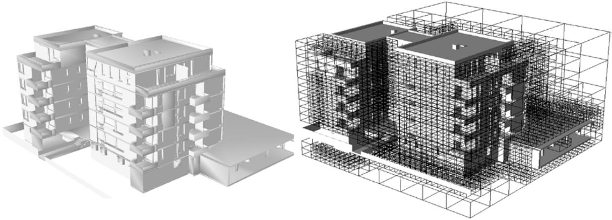
Figure 1: (a) Geometric representation of the building, (b) Deployed occupancy octree.
