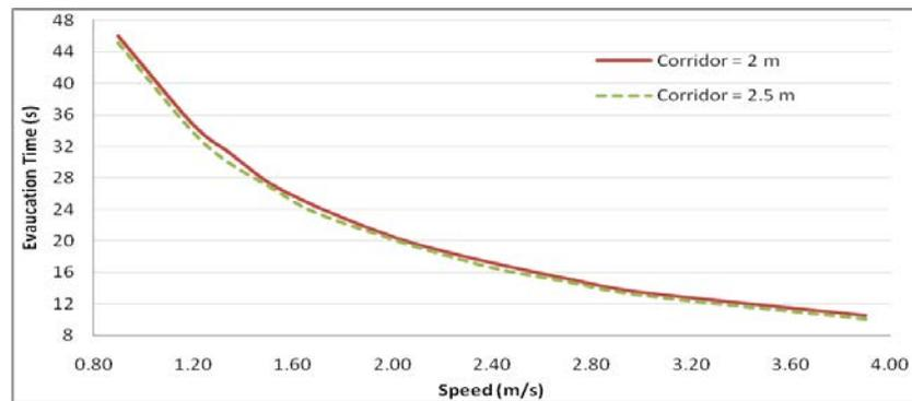
Figure 5: Evacuation time with various speeds (corridor = 2m, 2.5m)
