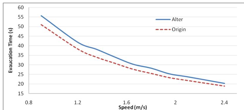
Figure 8: Evacuation times with original layout and alternative layout.
