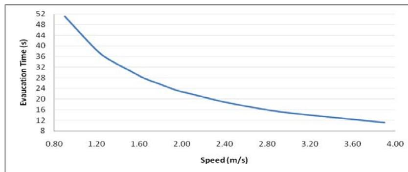
Figure 4: Evacuation time with various speeds (corridor = 1.5m)
