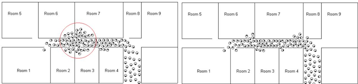
Figure 7: Congestion caused when doors are designed close.
