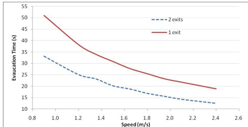
Figure 10: Evacuation time with using differets exits.
