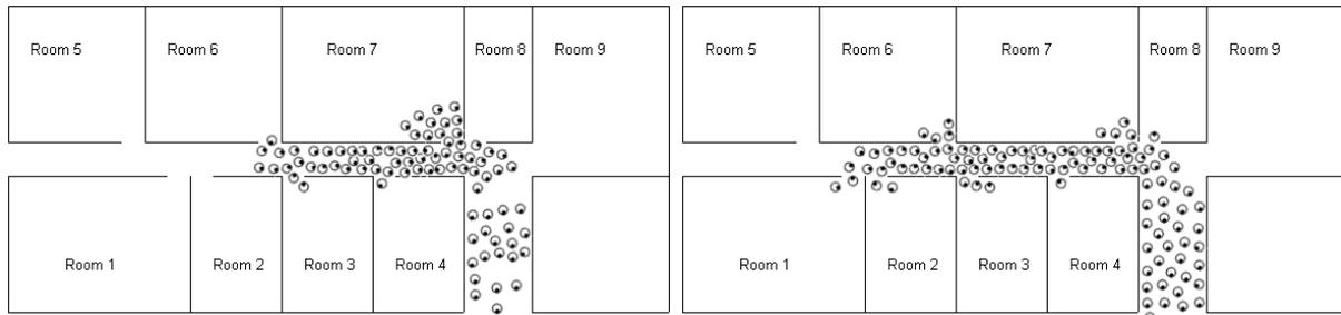
Figure 6: people speed: 0.9 m/s in room 7 (Left) and 1.5 m/s for the rest VS 1.5 m/s for all (right).
