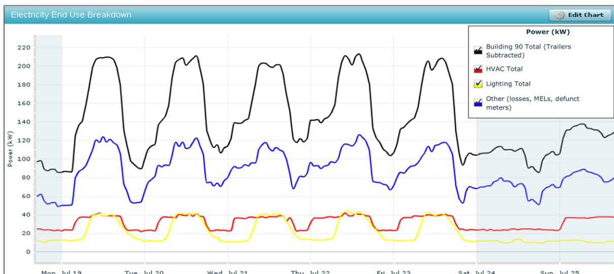
Figure 2 - Graphical comparison of HVAC, Lighting, and MELs in Building 90
